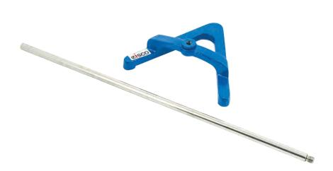
These sets are made from premium qulity metalware and built to provide maximum stability and durability. The bases are non ferrous cast iron with a high grade non toxic powdered coating and can be nested in one another for storage. The stainless steel rods have precise threading that results in a snug and stable fit into the bases.
